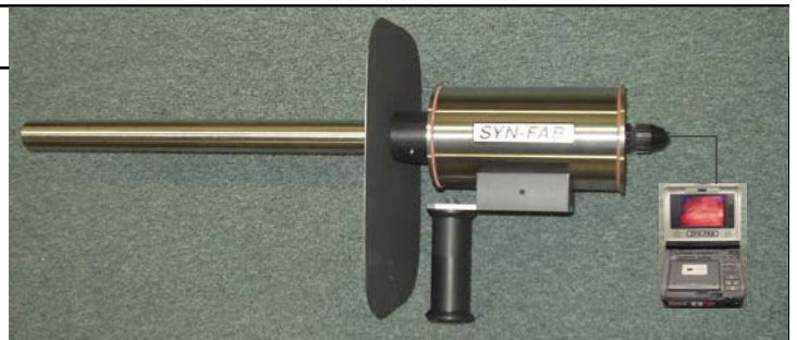
PORTABLE FURNACE INSPECTION SYSTEM
