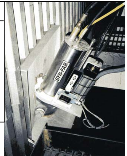
PERMANENT MOUNT SYSTEM WITH WALLBOX AND AUTOMATIC RETRACT
